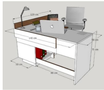
Figure 14. Recommendation 1 Multifunctional Work Desk
