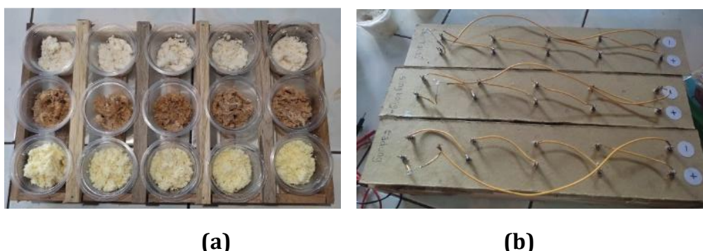
Figure 4: (a) measuring the voltage on the MFC circuit, (b) measuring the electric current
